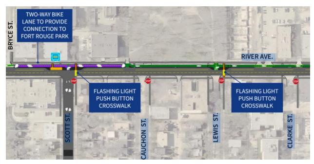
Proposed design for the River-Stradbrook protected bike lanes show how access between the Goulet bike lane and Braemar could be provided
