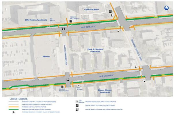
The pedestrian corridor crossing treatments proposed for the Enfield Cr crossings of Marion and Goulet are inadequate.
