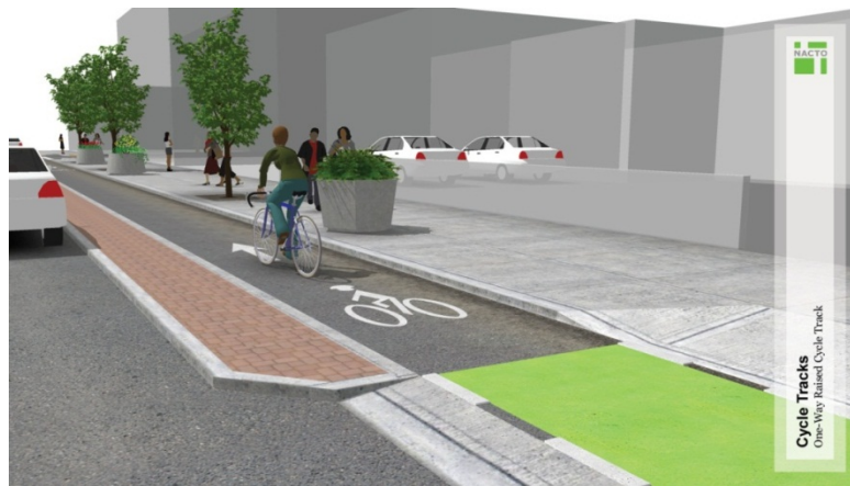
Illustration of Raised Cycle Track taken from the NACTO Urban Bikeway Design Guide
