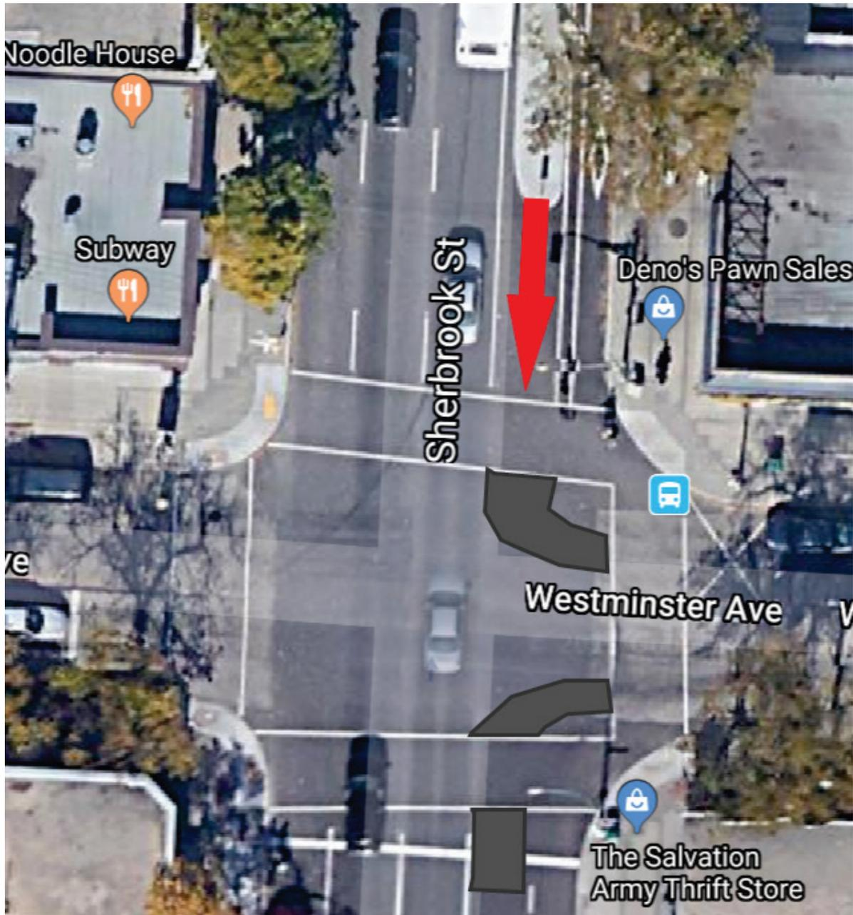
Protection for people on bikes needs to continue into the intersections to help facilitate turns and to keep everyone safe. Best practice for an intersection where protected bike lanes meet is for a protected intersection, which provides better separation between people on foot, on bike, or driving.
